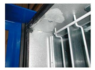
7. Remove the three 7/16 nuts and remove the three carriage bolts on the top hinge.
