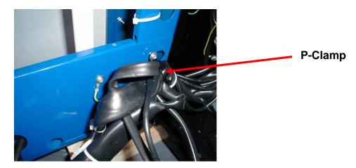
5. Remove the screw which secures the ground wire and pull the harnesses away from the door.
